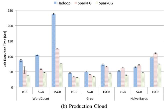
Fig. 2: Single Tenant Performance: Benchmark execution time in seconds for Hadoop and Spark on Mesos for different input sizes. In this experiment, we execute each job using Hadoop, Spark in coarse grained mode (SparkCG), and Spark in fine grained mode (SparkFG), using the development cloud (Figure 2a) and production cloud (Figure 2b).
