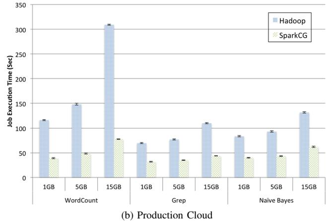
Fig. 3: Multi-tenant Performance: Benchmark execution time in seconds for Hadoop and SparkCG using different input sizes deployed on the development cloud (Figure 3a) and the production cloud (Figure 3b). In this setting, SparkCG receives offers from Mesos first because it is able to setup the application faster than Hadoop is able to.
