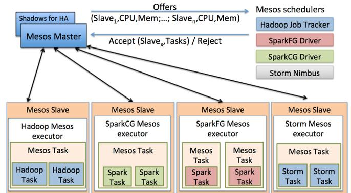
Fig. 1: Mesos Architecture. Each distributed computing framework implements a Mesos scheduler which negotiates with the Mesos Master for Slave resource allocation, and a Mesos executor inside which framework tasks are spawned. Frameworks launch tasks in Coarse-Grained (CG) mode (1 Mesos task corresponds to 1+ framework tasks) or Fine-Grained (FG) mode (1 Mesos task corresponds to 1 framework task). Spark can use either CG or FG modes; Hadoop and Storm use CG.
