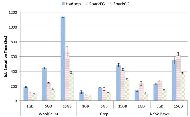
Fig. 8: Hadoop and Spark performance on Mesos-managed cloud shared with Storm: Execution time in seconds for Hadoop and Spark applications in CG and FG mode, for different input sizes and benchmarks on the development cloud.
