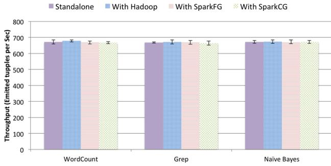
Fig. 9: Impact of Multi-tenancy on Storm in Mesos: When Storm receives its offers from Mesos ahead of the batch frameworks, there is no interference impact on Storm, i.e. Storm throughput is the same in multi-tenant and single tenant deployments.
