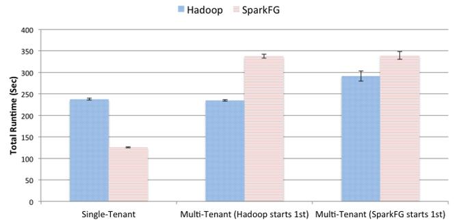
Fig. 6: Performance Implications of Multi-tenancy and Mesos Offer Order: Hadoop and SparkFG. This graph shows WordCount execution time in seconds for input size 15GB using the production cloud (single-tenant, multi-tenant with Hadoop ahead of Spark, and multi-tenant with Spark ahead of Hadoop).
