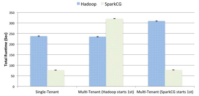
Fig. 5: Performance Implications of Multi-tenancy and Mesos Offer Order: Hadoop and SparkCG. This graph shows WordCount execution time in seconds for input size 15GB using the production cloud (single-tenant, multi-tenant with Hadoop ahead of Spark, and multi-tenant with Spark ahead of Hadoop). The framework that receives Mesos offers first performs best.
