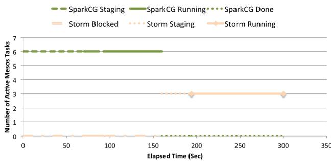
Fig. 10: Multi-tenant Interference between Storm and SparkCG in Mesos, broken down by stage of execution: When SparkCG receives its Mesos offers first, Storm blocks until SparkCG finishes.
