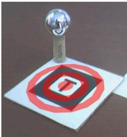
Figure 2: An ARToolKit marker with our light probe attached. The bullseye shows the marker has been recognized.
