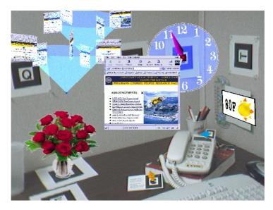
Figure 1: A typical ARWin desktop, as experienced through a video see-through head-worn display (Sony LDI-A55 with Point Grey Firefly camera). Applications are (clockwise from right) weather report, tagged phone, business card, flowers, web browser, clock.
