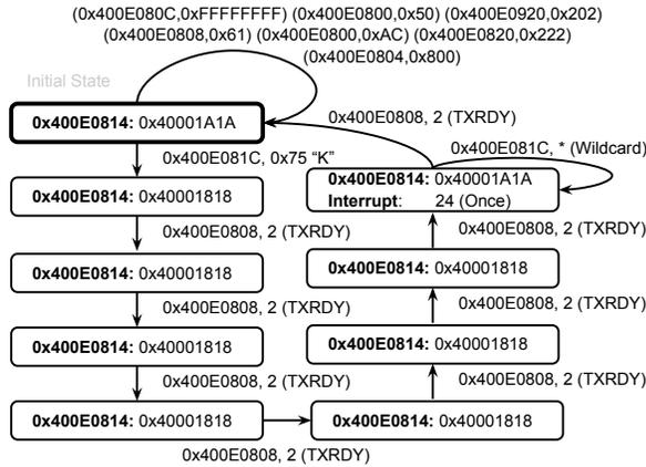
**Figure 5: An  $\omega$ -automata for a UART peripheral generated from a recording that prints “Knock!\r\n” repeatedly. The initial state will accept all configuration parameters, once a “K” is written, the peripheral becomes BUSY until the READY state is reached and interrupts are thrown.**
