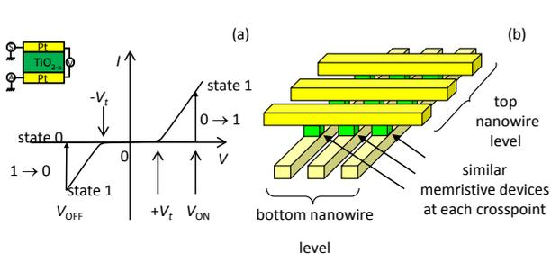
Figure 1: Crossbar memory: (a) I-V curve of a single memristor (schematically), (b) crossbar array structure
