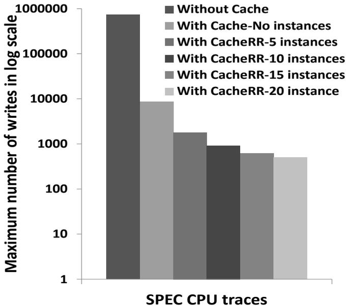
Figure 9: Effect of caching and distributed-sum scheme on the Maximum number of writes for SPEC traces. Cache size is 12KB
