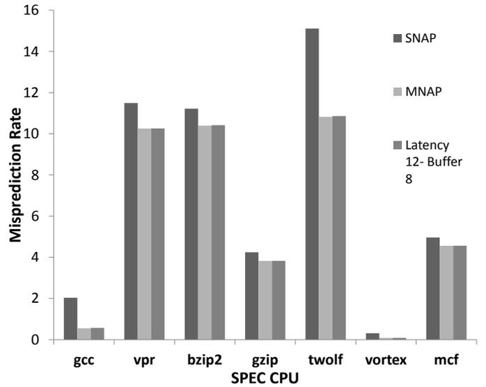
Figure 15: Misprediction rate assuming 12ns write latency
