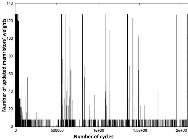
Figure 6: Number of weights evicted from SRAM to memristors. On average only 8 weights need to be updated
