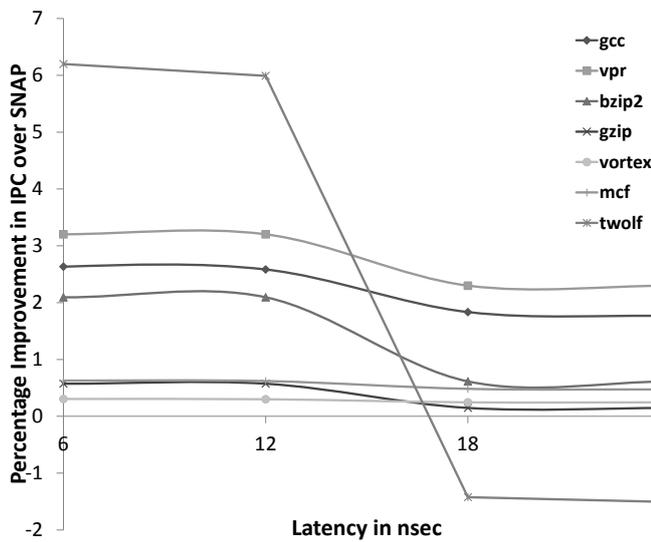
Figure 13: The effect of write latency on Performance
