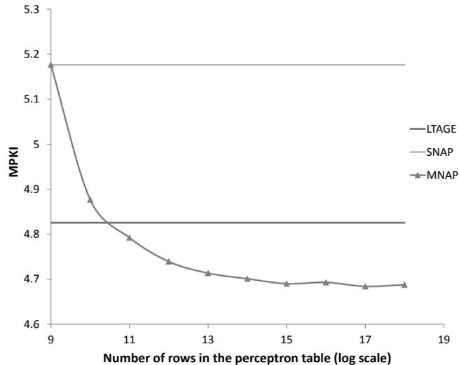
Figure 4: MPKI for SPEC CPU as the size of the perceptron table increase from  $2^9$  rows to  $2^{18}$  rows.  $2^9$  rows is the size of table in SNAP predictor
