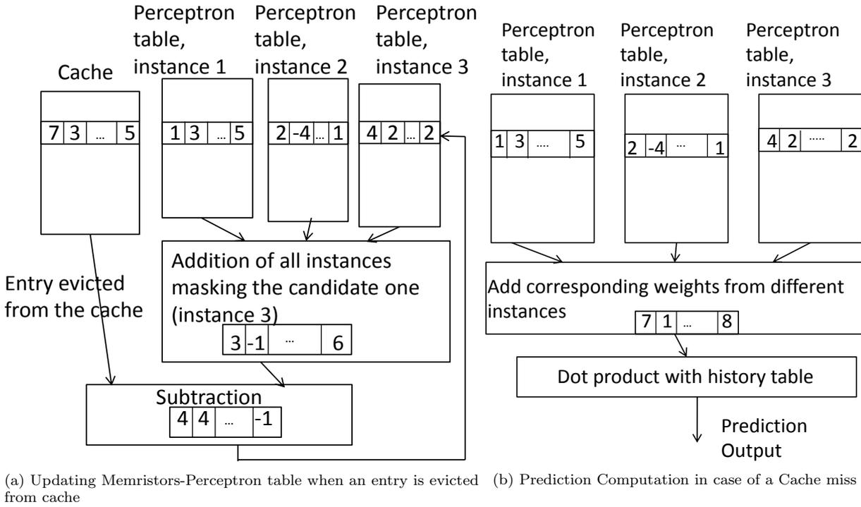
Figure 5: Weight update algorithm using Distributed-Sum technique and Prediction computation
