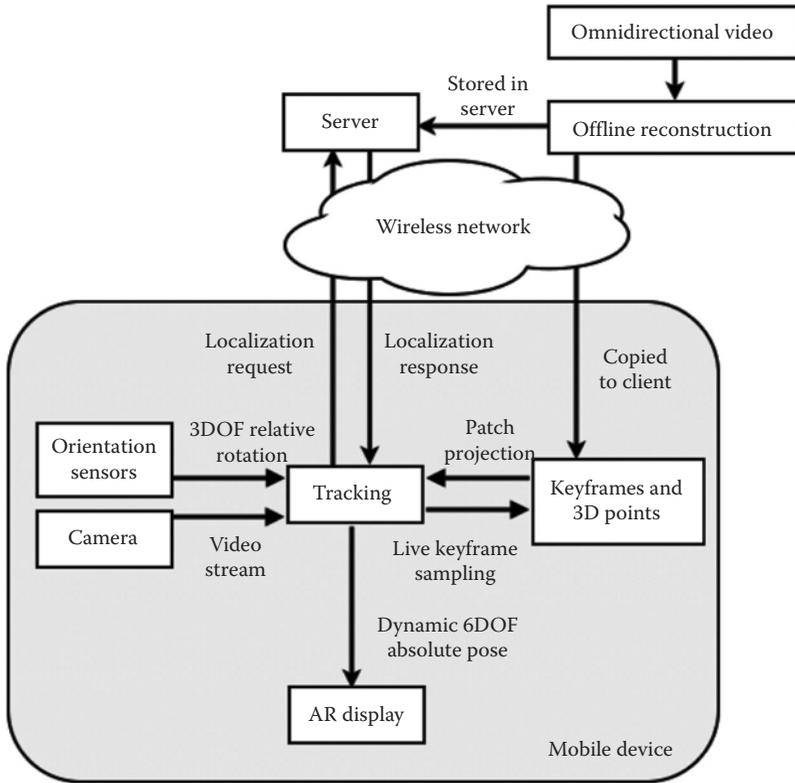
FIGURE 8.6 Tracking system overview with server/client design.
