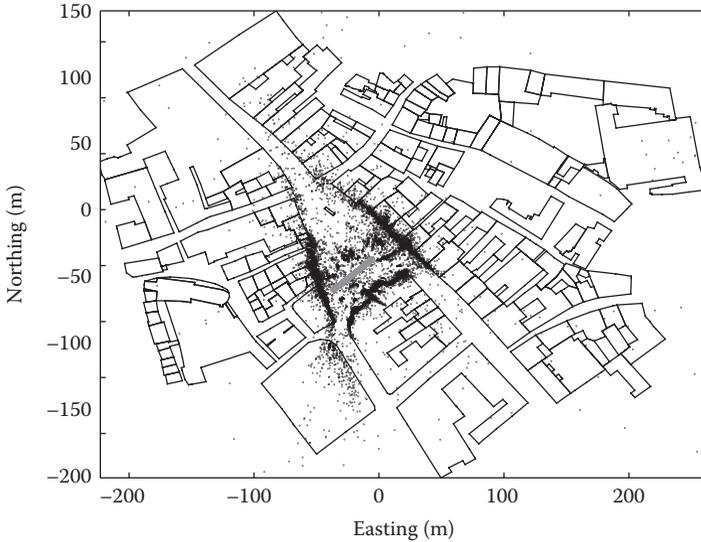
**FIGURE 8.5** Point cloud reconstruction aligned to OpenStreetMap building data. The gray dots indicate panorama capture locations, and the black points indicate triangulated 3D points.
