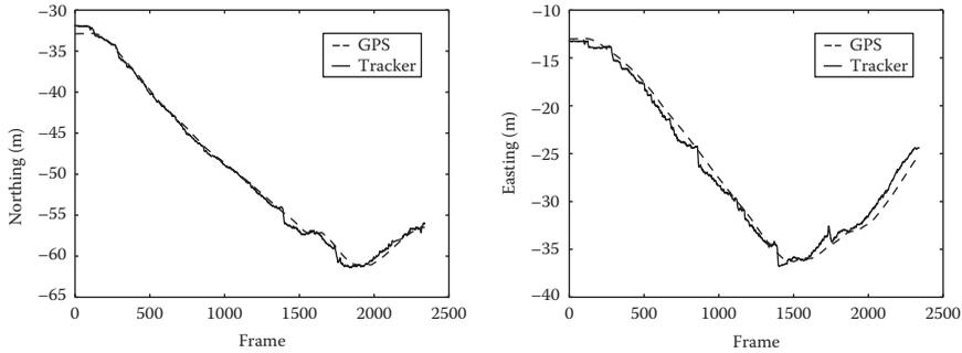
**FIGURE 8.7** Comparison of the camera position estimates from the visual tracking system with ground truth position estimates from the differential GPS receiver.
