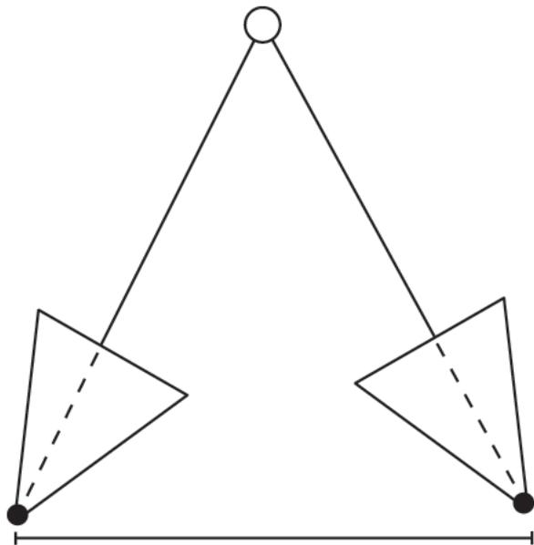
FIGURE 8.1 Triangulation of a 3D point from observations in two cameras. The distance between the cameras is called the *baseline*; the estimate is more accurate with a larger baseline.
