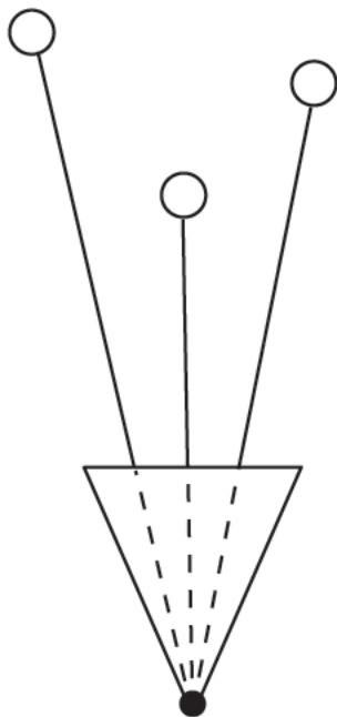
FIGURE 8.2 Localization of a camera from three 3D point observations. The estimate is generally more accurate when the points are nearer to the camera.
