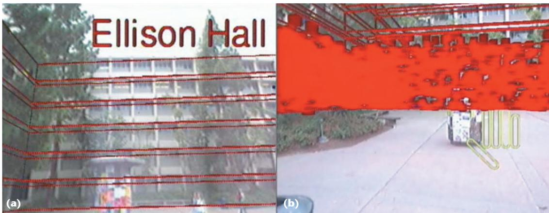
2 (a) Augmented reality view of one of the two buildings for which we built models. (b) Visualization of spots with "insufficient wireless" signal strength. The density of the data prohibits discerning differences in the data intensity.
